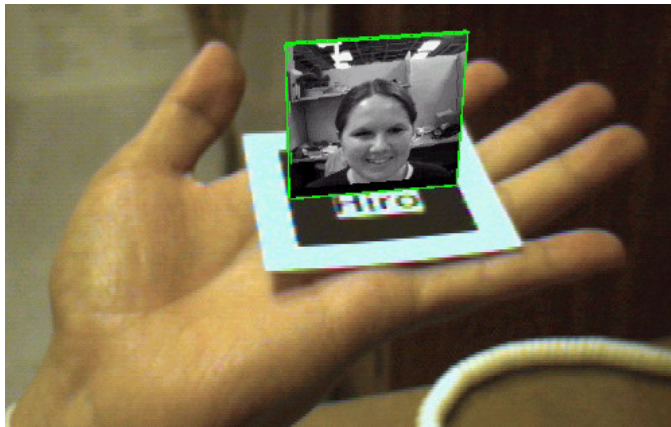
Image: Remote user representation in an augmented reality videoconference (Source: Kato et al [82]).
